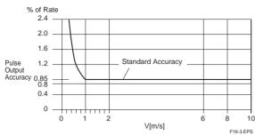
Current Output: Pulse output accuracy plus ±0.05% of Span **Repeatability:**
